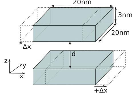
**Figure 1.** Schematic drawing of the InAs DQD cuboidal system. The dimensions of the QDs and the variable parameters  $d$  and  $\Delta x$  are indicated. The boxes with dashed lines represent the DQD with misalignment.
