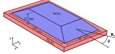
Fig. 1. Schematic representation of the uncapped InAs QD system. The dimensions of the QD considered in the simulations and the orientation of the magnetic field are also indicated. The upper base of the pyramid is 0.6 times the lower one.
