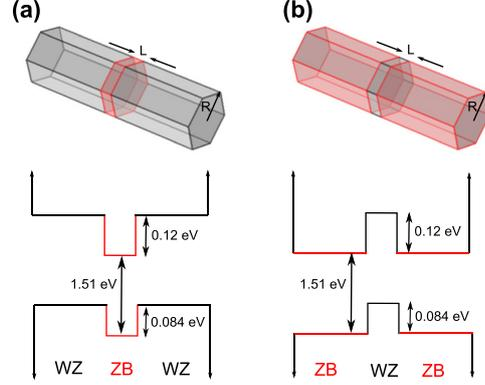
FIG. 1. (a) Sketch of ZB QD embedded in WZ wire and corresponding band-offset profile. (b) Same but for WZ QD embedded in ZB wire.
