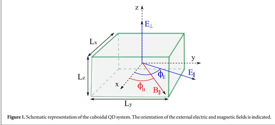
Figure 1. Schematic representation of the cuboidal QD system. The orientation of the external electric and magnetic fields is indicated.
