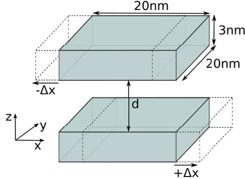
**Figure 4.10:** Drawing of the DQD cuboidal system. The dimensions of the QDs and the variables corresponding to interdot barrier thickness,  $d$ , and the shift in opposite directions along the  $x$  direction,  $\Delta_x$ , are indicated. Dashed lines represent the DQD with misalignment.
