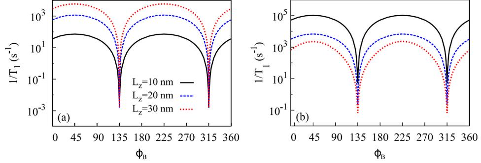
**Figure 4.9:**  $1/T_1$  versus  $\phi_B$  in square QDs grown along the [111] crystallographic direction. Simulations considering (a) pure RSOI and (b) pure DSOI are presented for three dot heights:  $L_z = 10$  nm (black solid line),  $L_z = 20$  nm (blue dashed line), and  $L_z = 30$  nm (red dotted line).
