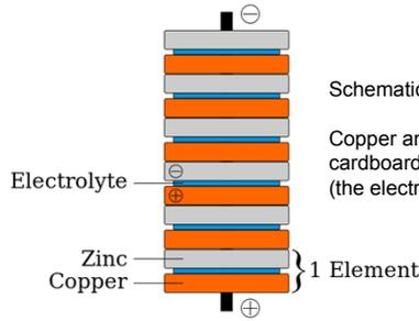
Schematics of a [copper-zinc](#) voltaic pile.
